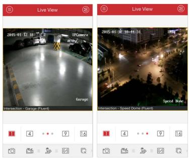
You can drag and move the window to adjust the window sequence. You can double-click the live view window to display the camera in 1-division mode and double-click again to restore.
