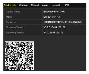
• iVMS-4200 (V2.3.0.4 or above): In the Device Management module, select Server tab, click to select a device and click **QR Code** to pop up the QR code window of the device.
